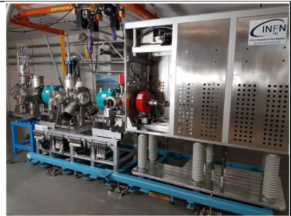
Figure 32 - Source protons de l'ESS [26] , 6 ms, 14 Hz
