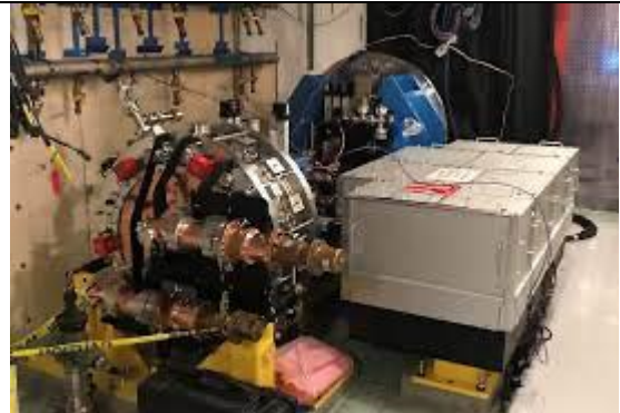
Figure 30 - Canon photocathode LCLS-II [24] , 1-100 fs, 1 MHz
