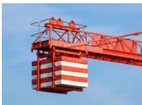
Figure 47 - Contre-poids de grue
